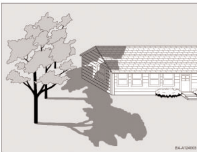
Locate trees to shade the east and west windows and walls. As trees mature, they will shade your roof, too.
